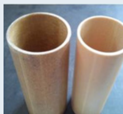
3. PVC/keratin fibre composite
