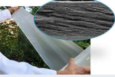
Figure 1. CNF film with micropatterned surface. ting Pillars with a diameter of 7.5  $\mu$ m d a height of 1.5  $\mu$ m were printed.
