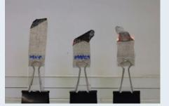
Figure 2: Flammability test on treated (left and middle) and non-treated (right) flax fibre fabrics [2]
