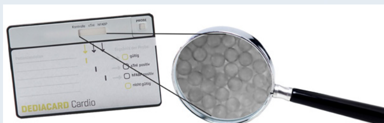
Figure 2. "Dediocard Cardio" rapid test for detection of heart attack based on nanostructured polymer membranes.
