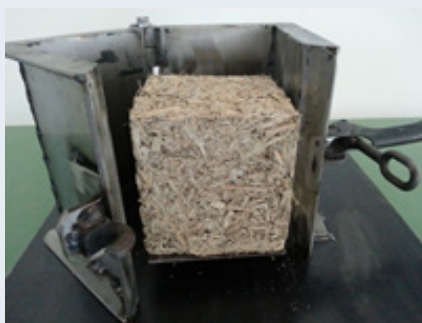
A freshly prepared concrete bloc made with miscanthus stem fragments.
