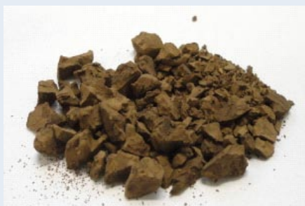
Fig. 1 Sulphur free lignin obtained after extraction using hydrotropic solution and precipitation in water. A simple and sustainable way to disassembly lignin from biomass.
