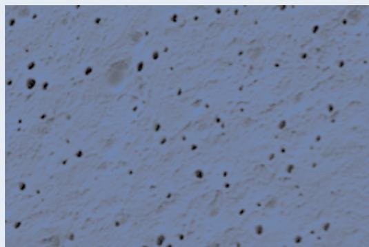
Fig. 2: HDL-LS 1%-reinforced starch particles (0.5µm diameter) dispersed in polyethylene
