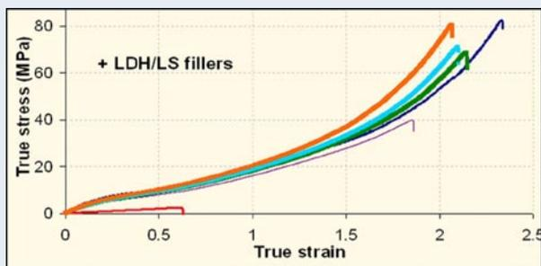
Fig. 2: Stress-strain curve for LDH/LS filled thermoplastic starch concentrated at 20% in polyethylene (PE). Blue: pure PE. Red: pure starch, pink: unfilled starch-PE. Other curves LDH/LS based blends with content of LDH/LS of 1, 2, and 4%.
