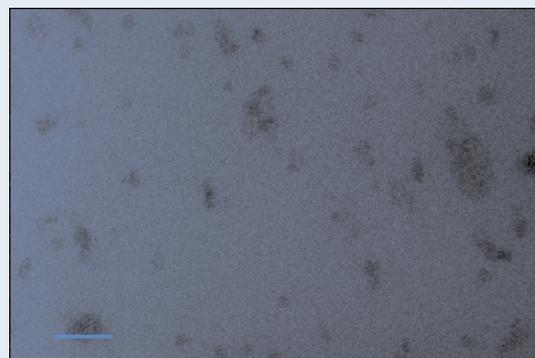
Fig. 1: LDH/LS dispersed in starch at 1% concentration seen by transmission electron microscopy. The white bar represents 100 nm.
